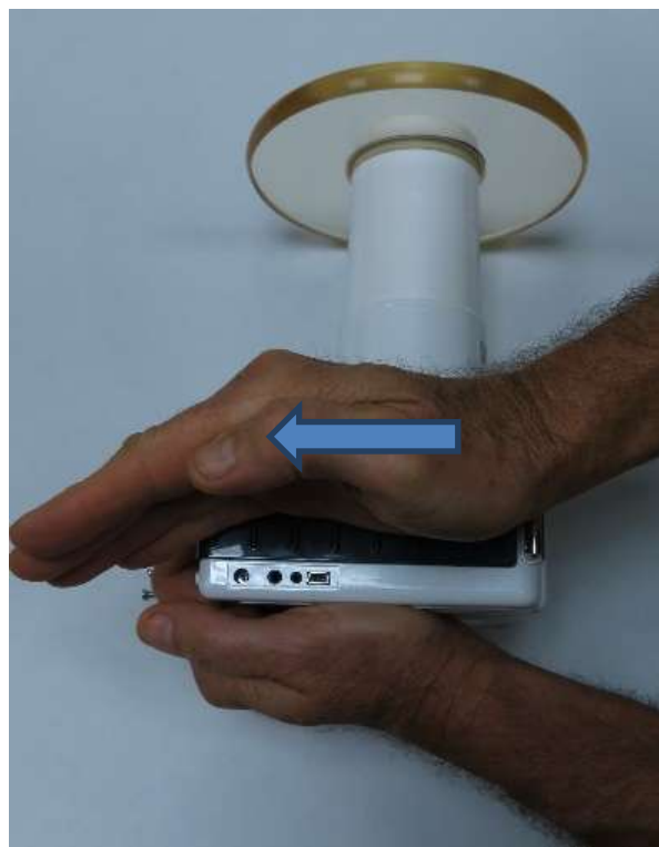
Figure 2 - Slide side cover towards bottom
