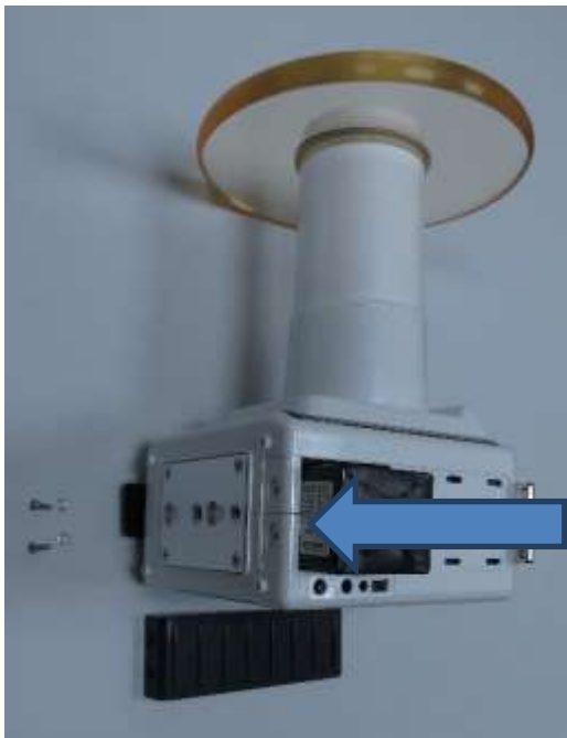
Figure 4 - Battery partially removed, showing correct orientation with CE mark towards bottom of body
