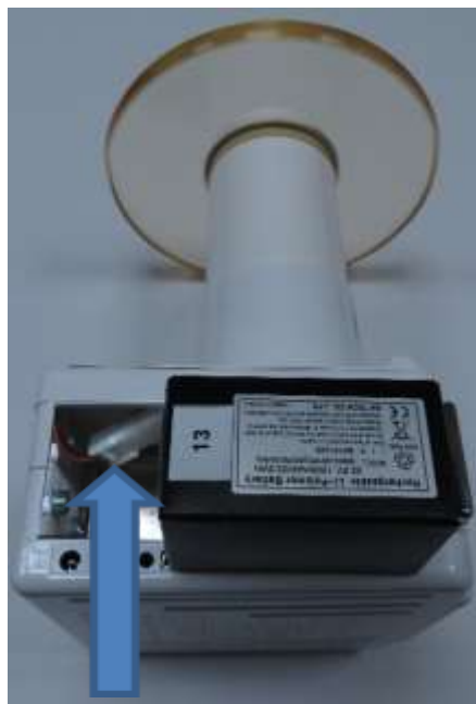
Figure 5 - Battery plug tucked into front of body
